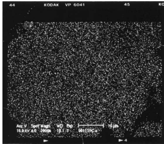
Fig. 5. Ca K \alpha X-ray map of a fresh lime particle.
